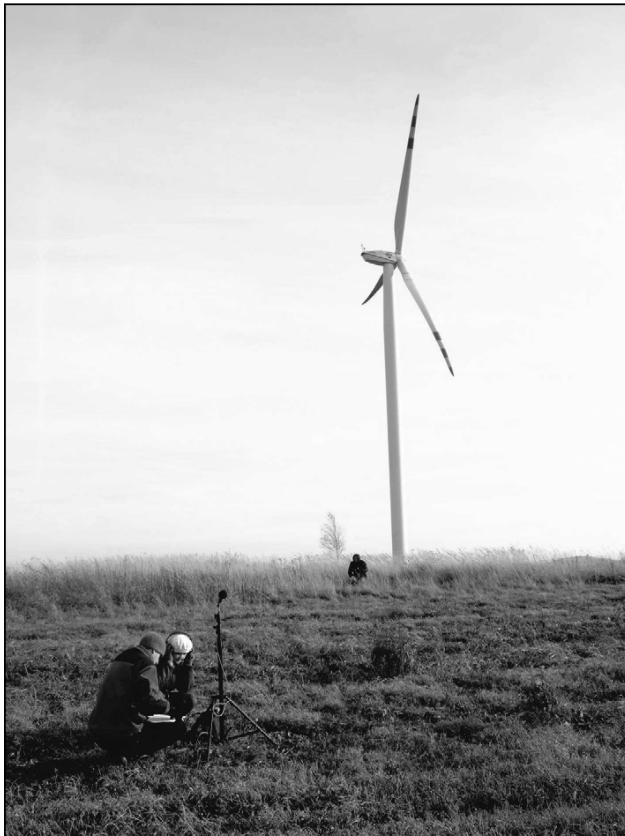
Fig. 9. Acoustic measurement of REpower M92 wind turbine in the village Lęki Dukielskie (own photo).
