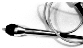
Fig. 7. A fabricated thermal sensor based on SAW.
