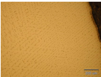
Fig. 2. The dendritic microstructure developing from the casting surface in Co-Cr-Mo-W alloy
