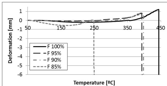
Fig. 7. Hot distortion research of moulding sand mixtures with different content of furfuryl resin
