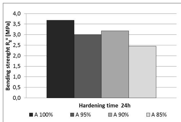
Fig. 6. Bending strength of moulding sand mixtures with different content of alkyd resin
