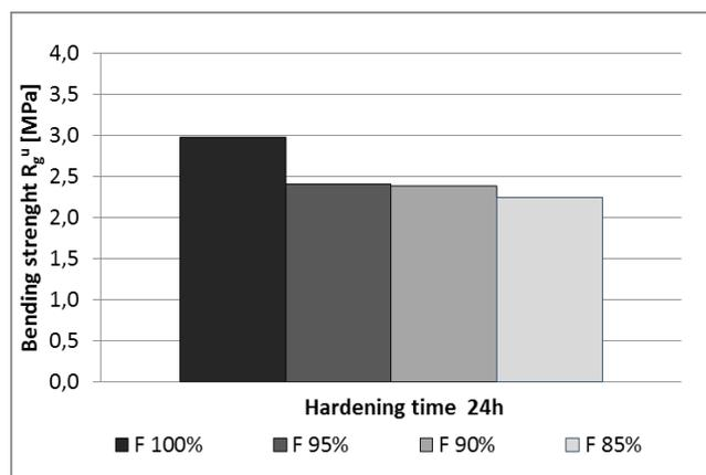
Fig. 4. Bending strength of moulding sand mixtures with different content of furfuryl resin
