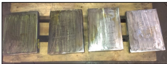
Fig. 9. Polished castings prepared for ultrasonic testing
