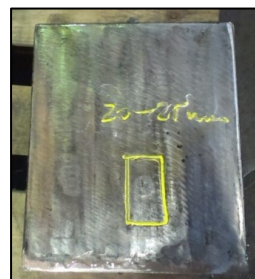
Fig. 10. The position of shrinkage cavity
