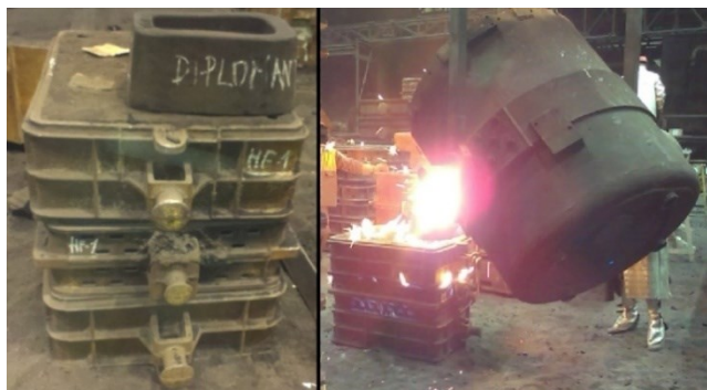
Fig. 7. The completed mould No.1 and pouring
