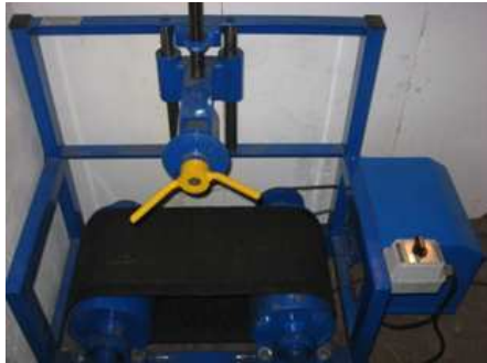
Fig. 1. The measurement station of the acoustic emission testing of tires.
