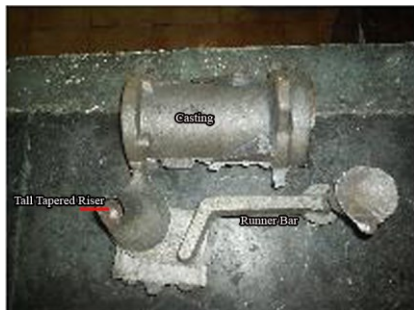
Fig. 4. Casting with redesigned feeding system
