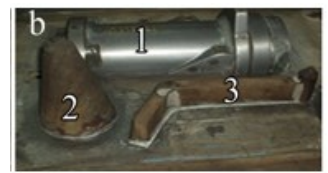
Fig. 3b. Cope pattern - modified design
