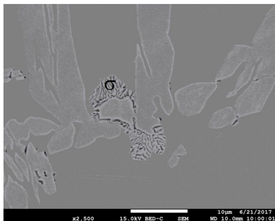
Fig. 3. BSE image of material „1”– the \sigma phase
