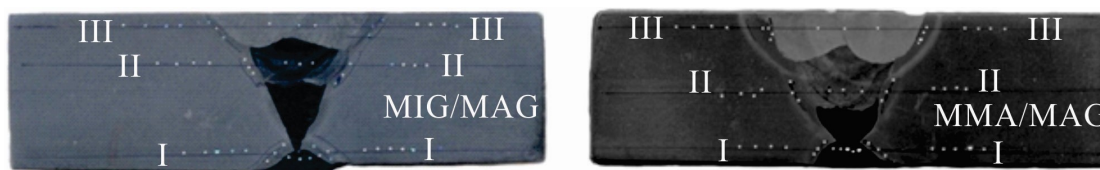
Fig. 2. Metallurgical samples of MIG/MAG and MMA/MAG welded joints with directions and positions of microhardness measuring
