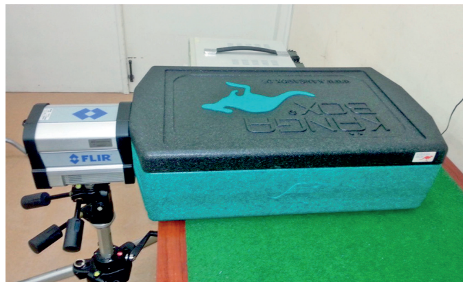
Fig. 17. External view of thermal resistance testing stand
