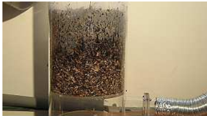
Figure 4: Dew point occurrence in the packed bed.
