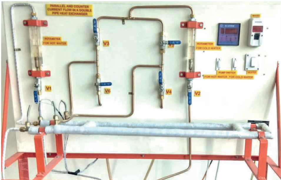
Fig. 1. Experimental set-up of tube in tube heat exchanger
