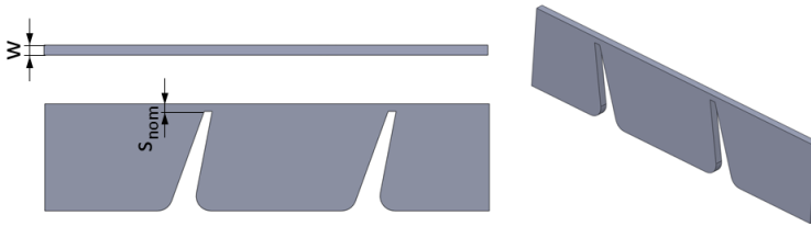
Fig. 4. Labyrinth seal geometry
