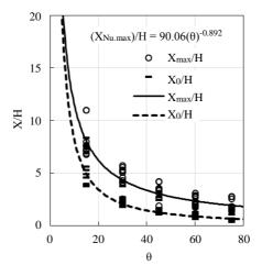
Fig. 9. Variation of  $X_{\text{Nu,max}}$  and  $X_0$  – related with jet inclination
