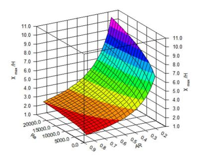
Fig. 7.  $X_{\text{Nu.max}}$  – variations between Reynolds Number (Re), target to jet height (H), and Angle Ratio (AR)
