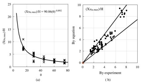
Fig. 8. Equation suggested for  $X_{\text{Nu.max}}$ : a) variation w.r.t. jet inclination angle b) comparison with experimental and equation results
