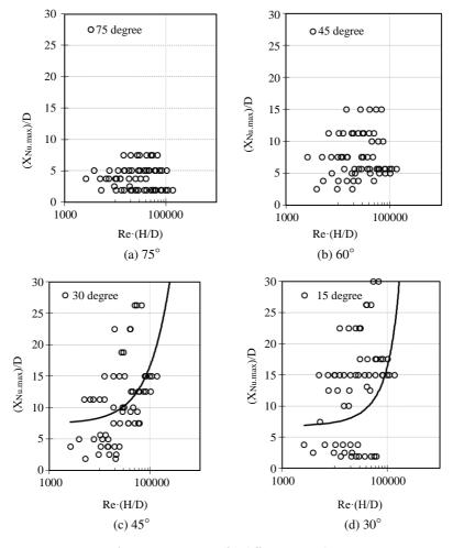
Fig. 6.  $X_{\text{Nu,max}}$  positions for different jet inclinations
