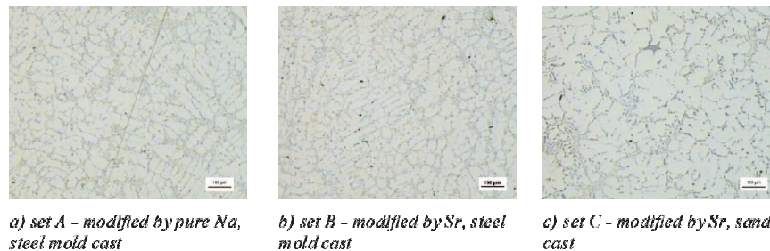
Fig. 1. Typical microstructure of AlSi7Mg aluminum cast alloy
