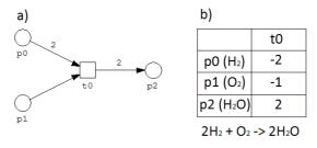
Figure 1: a) A graphical representation of a simple Petri net modeling synthesis of water; b) an incidence matrix of the net presented in part a).
