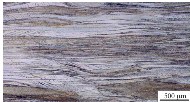
Fig. 1. Microstructure of the HE copper, \varepsilon = 2.24 ; longitudinal section of the sample
