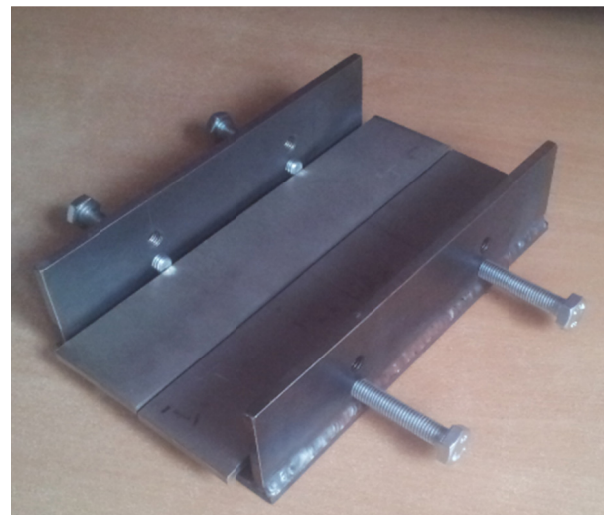
Fig. 3. View of plates after sand blasting. From the left: 6 plates, 10 R_a in roughness, 6 plates, 5 R_a in roughness and 6 plates, 1 R_a in roughness
