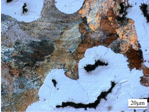
Fig. 5. The microstructure of the CGI containing 1.47% Ni in castings with the wall thickness of 24 mm: compacted graphite, pearlite, ferrite
