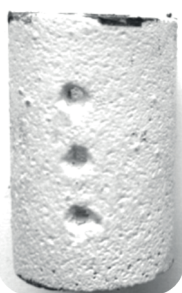
Fig. 2. Sample covered by zirconium coating to ultrasonic investigations
