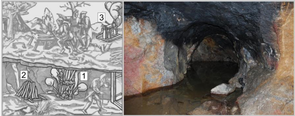
Fig. 3. Principle of fire-setting (according Agricola, 1556): (1) kindled logs, (2) heap of dried logs, (3) fumes ventilation; photo illustrates an example of the rest of soot on the roof of gallery ( photo: Lednická )
