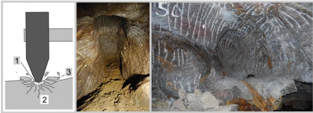
Fig. 2. Principle of rock ruptures after hammer blow (according Lehrberger & Gillhuber, 2007): (1) crushed zone, (2) cracked zone – radial cracks, (3) abruption of fragments; photos illustrate examples of mined out spaces using hammer blow in the Jeroným mine ( photo: Lednická )
