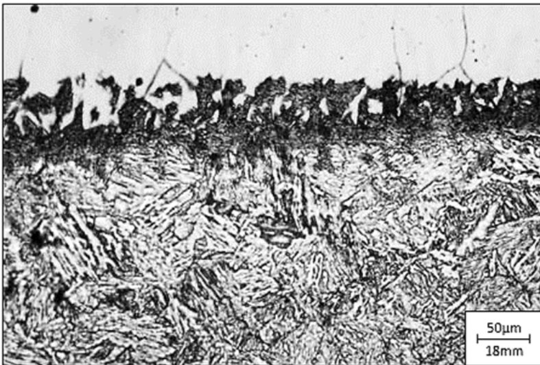
Fig. 13. Martensite micro-structure of original material with visible welding line
