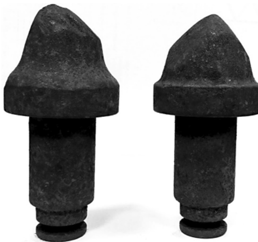
Fig. 7. Tangential-rotary picks with broken cutting edge during exploitation
