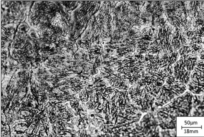
Fig. 12. Martensite microstructure of the padding weld made with use of electrode ABRADUR54
