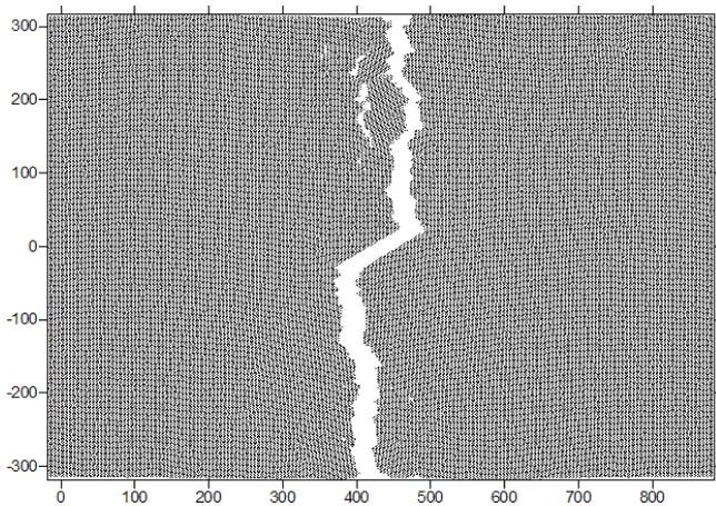
Fig. 4. Deformation at extension 4.1%
