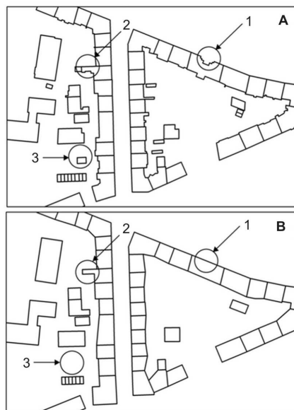
Fig. 2. Recognizability of buildings generalized from the scale 1:500 to the scale 1:10 000 (scale of the presentation 1:2000): A – original data, B – data converted to the scale 1:10 000;
