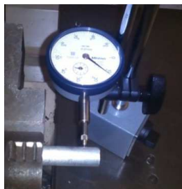
Fig. 16. Runout measurement using a dial indicator.
