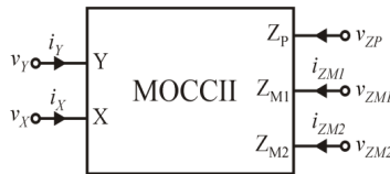
Fig. 1. A graphic symbol of the proposed multiple output second-generation current conveyor (MOCCII) block.
