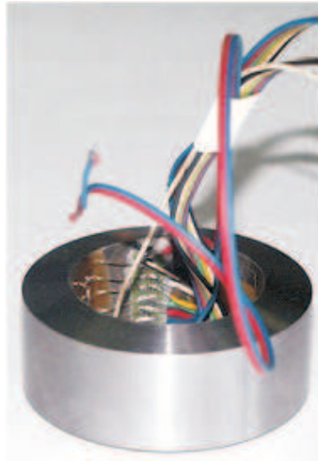
Fig. 8. The examined gasket with fixed gauges
