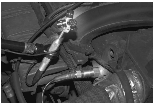
Fig. 17. Microphone recording an acoustic signal of the car engine operation
