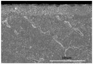
Fig. 6. The microstructure of the AgCu6Ge1 alloy, 500x
