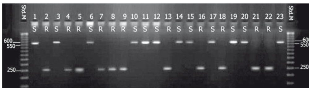
Fig. 3. SCAR marker HVS3 patterns of 23 barley varieties. Upper band (575 bp) susceptible lines, lower band (250 bp) resistant lines. From left to right, standard ladder (50 bp), 1 = Tadmor, 2 = H. spontaneum 41-1, 3 = H. spontaneum 41-1/Tadmor (1), 4 = Hml (Union/C103576/Coho), 5 = WI2291, 6 = SLB05-96, 7 = Zambaka (Pure line from Arabi Aswad), 8 = SLB45-40/ H. spontaneum 41-5, 9 = H. spontaneum 41-5, 10 = SLB39-39, 11 = Arta, 12 = Arabi Abiad/Arar, 13 = Sara (Arar/Arabi Aswad, 14 = H. spontaneum 41-1/Arta, 15 = SLB39-01, 16 = Moroc9-75, 17 = Moroc9-75/ H. spontaneum 41-1/Tadmor, 18 = Moroc9-75/ Arabi Aswad, 19 = Clipper, 20 = JLB37-74, 21 = Harmal-2, 22 = Sel160, 23 = Rihane-2, standard ladder (50 bp). Varieties 19 and 23 were used as a susceptible control
