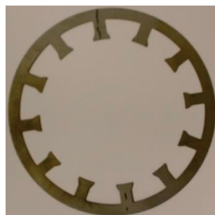
Lamination of outer stator steel
