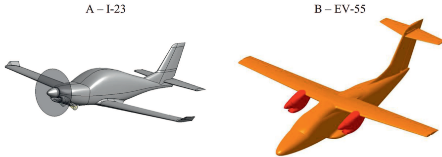
Figure 1: Airplanes: A) single-engine I-23 with the engine in the fuselage and B) twin-engine EV-55 with engines on the wings.
