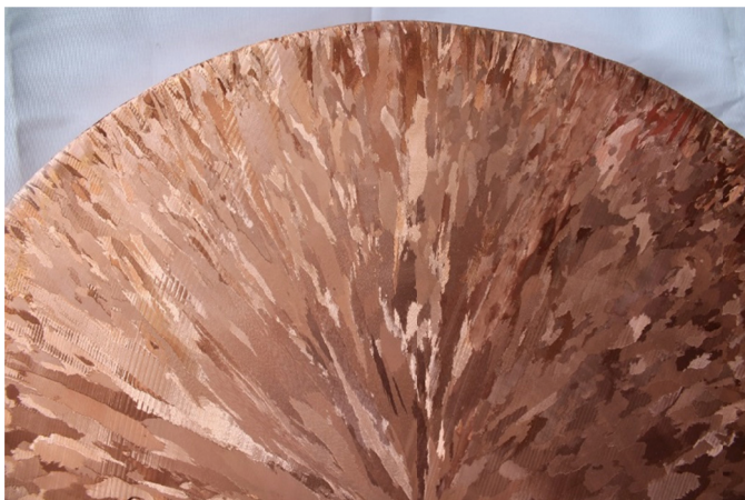
Fig. 3a. Two types of columnar (FC – fine columnar and C – columnar) structure revealed on the brass ingot cross-section
