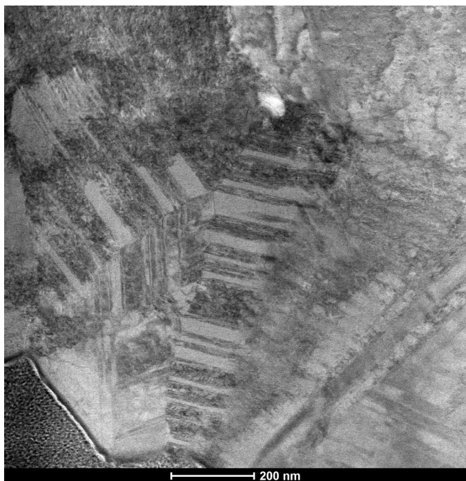
Fig. 6. STEM-BF image of the cross-section of a Cu/Ni multilayer system (substrate with copper and nickel layers)
