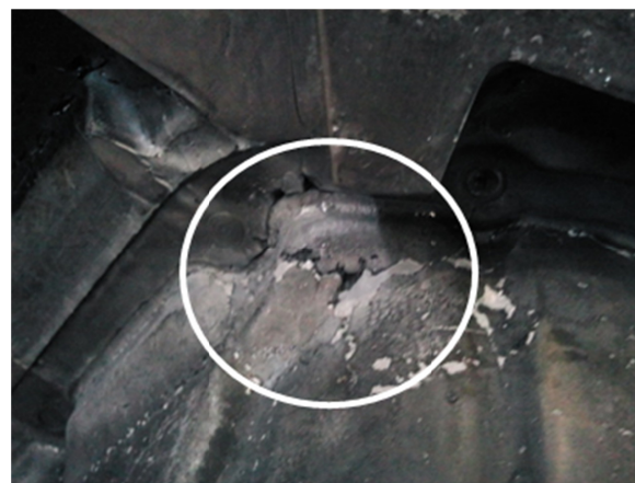
Fig. 3 Photograph of the damaged portion of the die
