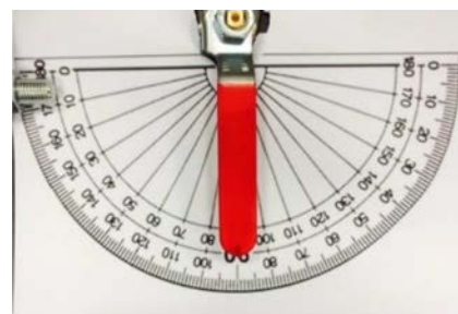
Fig. 3. Protractor instrument for measuring angles at suction valve of the pump.
