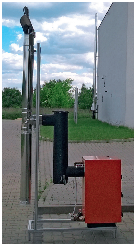
Jabłonna Research Center – demo version of an electrostatic filter together with a boiler.
