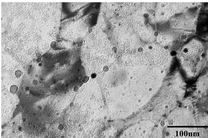
Fig. 4. Oxide particles on the grain boundaries in ODS ferritic stainless steel with Hf addition
