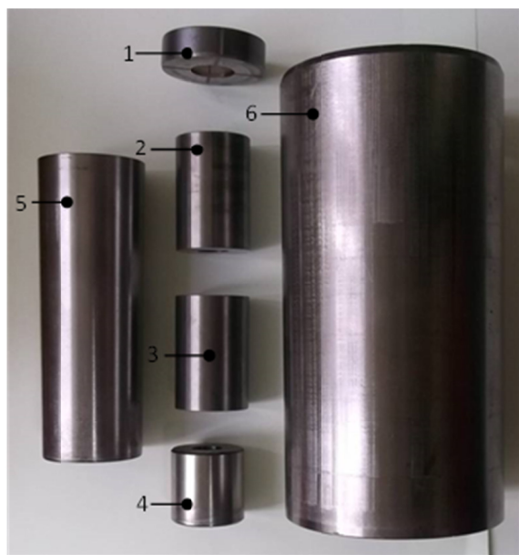
Fig. 3. The components of the tool die shaping operation for the fourth bolt: 1 – die, 2, 3, 4 – spacer sleeve, 5 – the centering tube blank, 6 – casing
