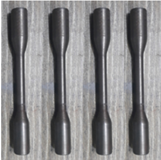
Fig. 6. a) Tensile test specimen as per ASTM standard and b) Stress Vs Strain curve for ADI
