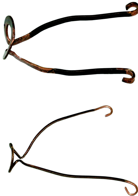
Fig. 21. Deformation of coil in compressing inductor
