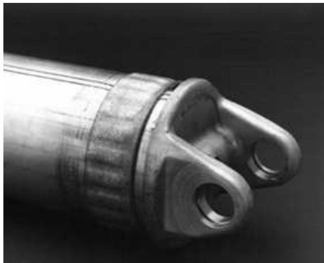
Fig. 3. Fitting of an aluminum drive shaft using the electrodynamic method
