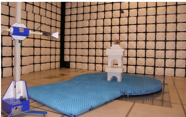
Fig. 5. Example of the test setup for radiated emissions measurement above 1 GHz in the SAC of WUST EMC laboratory
