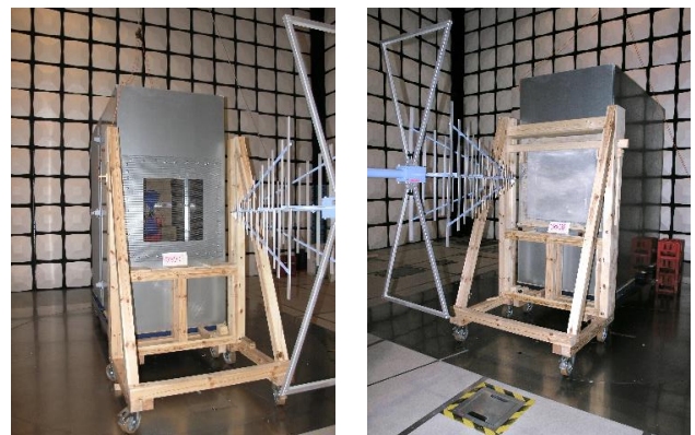
Fig. 42. An example of the test setup used for shielding effectiveness measurement of steel mesh (left) and block of concrete (right) in the SAC
