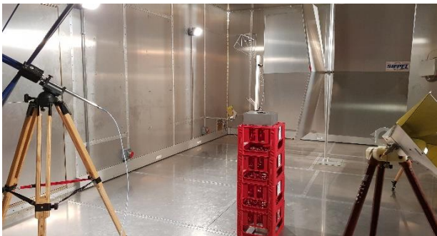
Fig. 3. Example of the test setup with the SAC in WUST EMC laboratory
