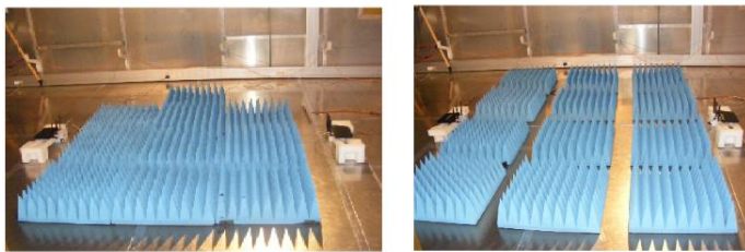
Fig. 19. Example of 12 absorbing panels installed on RC's floor: left) grouped (N=12 in fig. 18), right) separate (N=13 in fig. 18)
