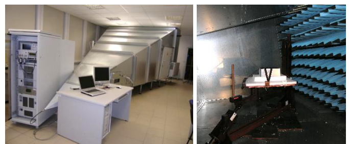
Fig. 4. Example of the test setup for radiated emissions measurement in the GTEM cell of WUST EMC laboratory and GTEM's interior with manipulator and installed EUT
