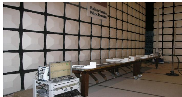
Fig. 7. Example of the test setup for conducted emission with use of current probe according DO-160G [22] in the SAC of WUST EMC laboratory
