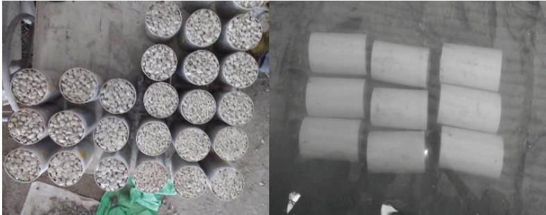
Figure 1. Pervious concrete specimens
