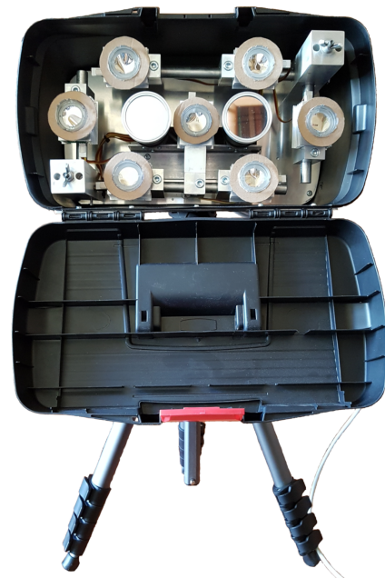
Fig. 3. View of the measurement system for medical imaging and diagnostics, for the continuous and stroboscopic mode (utility model No. W.127607).
