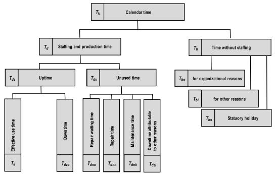
Fig. 3. Division of calendar time with the built-up automated system Source: own study based on (Lisowski 2001)
