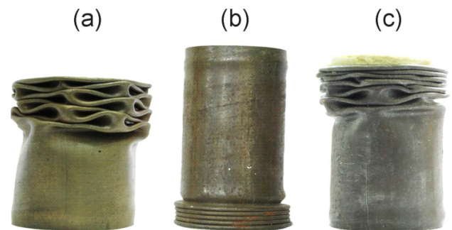
Fig. 4. Typical collapse modes of single-walled and double-walled tubes: a – diamond (asymmetric), b – concertina (axisymmetric), c – mixed
