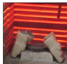
Fig. 3. Firing of moulds in resistance heating furnace
