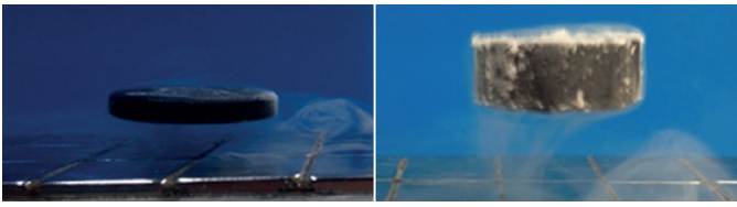
Fig. 8. The influence of levitation force on two different superconductors
