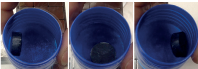
Fig. 9. The influence of force and torque resulting from flux pinning effect
