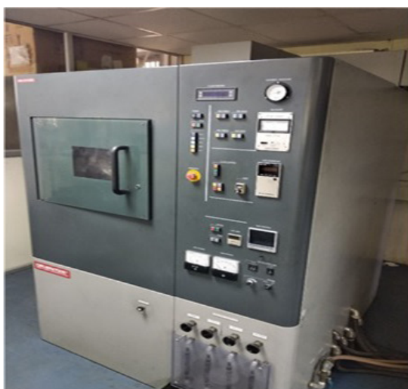
Fig. 2. Photosnap of the SPS machine and prepared composite
