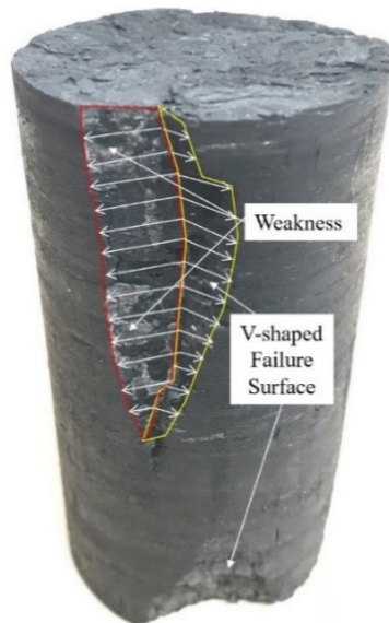
Fig. 8. Fracture surface formed after ejection
